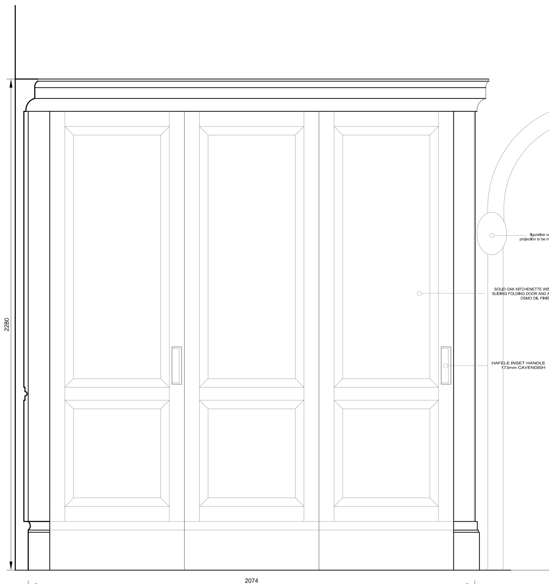
1:10 FRONT ELEVATION OF KITCHENETTE (Doors Closed)
